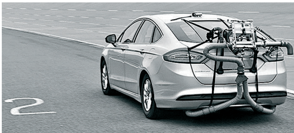
Rys. 15. System PEMS do badań emisji spalin w warunkach drogowych (autoevolution, 2019) Fig. 15. PEMS system for testing exhaust emissions in road conditions (autoevolution, 2019)
