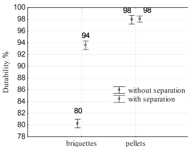
Fig. 3. Interaction of fuel forms with the separation of particles on the mechanical durability of briquettes and pellets made from miscanthus
