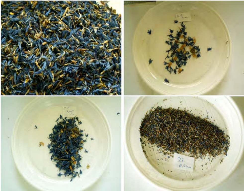
Figure 4. Example of selected fractions of the mixture subject to pneumatic separation
