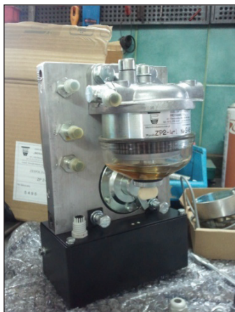
Figure 1. Measurement unit a – flow meter ZP@-4-I by Rotameter company, b – NOSAL-TECH mounted on a tractor
