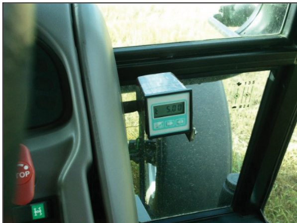
Figure 1. Measurement unit a – flow meter ZP@-4-I by Rotameter company, b – NOSAL-TECH mounted on a tractor
