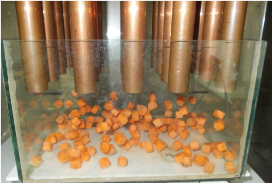
Figure 4. View of the bed of carrots cubes under fluidization
